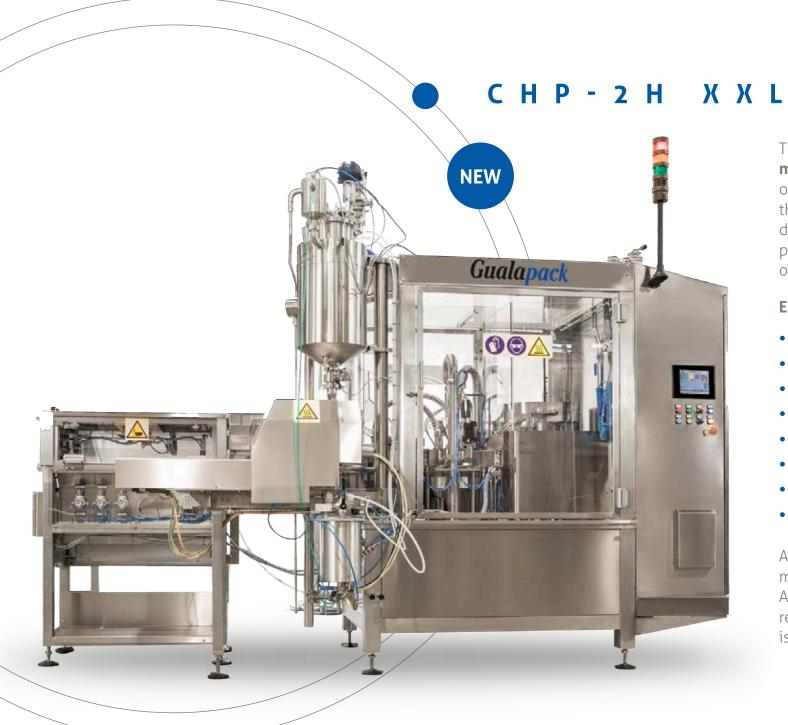
The CHP-2H XXL has been built to satisfy **medium** filling annual volumes, based on a step by step rotating table on which the pouches are filled and capped, it's designed for packing liquid or viscous products into various sizes of pre-made pouches.
